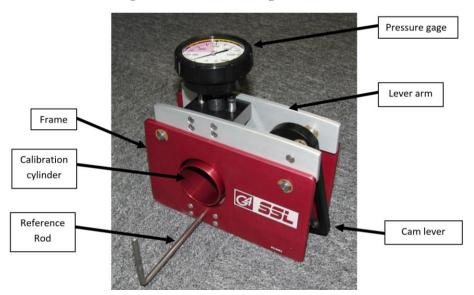
Step 1: Insert a softball bat through the 2.5" diameter hole in the frame until the end of the barrel touches the reference rod (also place the calibration cylinder between the handle of the bat and the table to keep the bat level with the fixture).
