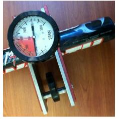
Step 2: Apply a preload by rotating the pressure gage clockwise until the gauge reads 500psi for the USA version or 0 lbs for the universal version. This will ensure good contact with the bat and the anvils. Make sure the cam lever is in the full down/vertical position.
