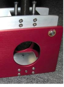
Step 2: Hand tighten the setscrew to ensure the reference rod does not rotate.
