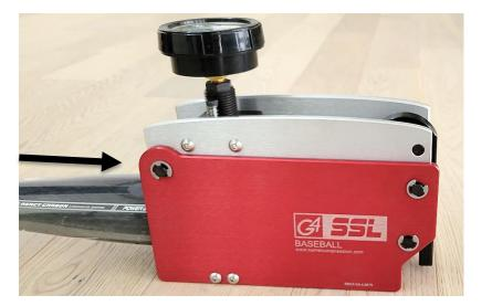
**Step 1**—Insert a baseball bat (2-5/8" barrel diameter) through the open end of the frame until the end of the barrel touches the bat stop. Be sure to push the black cam lever down to the frame until it stops and is vertical.
