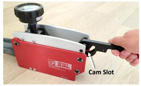
**Step 3**—Pull the cam lever up to the horizontal position until it seats and stops. The force that is read on the gauge is the barrel compression.
