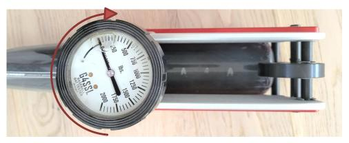
Step 2— Turn the gauge clockwise to preload the bat until the needle reaches0 lbs. As you are preloading, be sure the cam lever stays down, and is vertical.Be sure the endcap of the bat is touching the bat stop.
