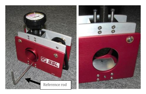
Step 2: Hand tighten the setscrew to ensure the reference rod does not rotate.
