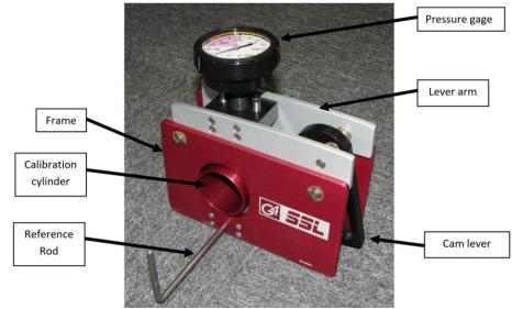
Step 1: Insert a softball bat through the 2.5" diameter hole in the frame until the end of the barrel touches the reference rod (also place the calibration cylinder between the handle of the bat and the table to keep the bat level with the fixture).
